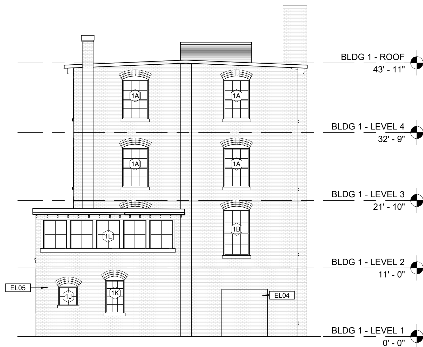
21 BLDG 1 - EAST ELEVATION Scale: 1/8" = 1'-0"
